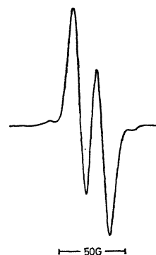
Fig. 1. ESR spectrum of \gamma -irradiated silk, measured at room temperature.
